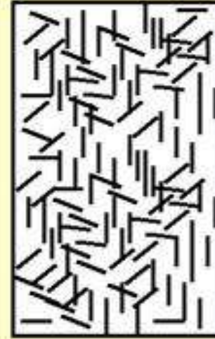
Discontinuous and randomly oriented fibers
