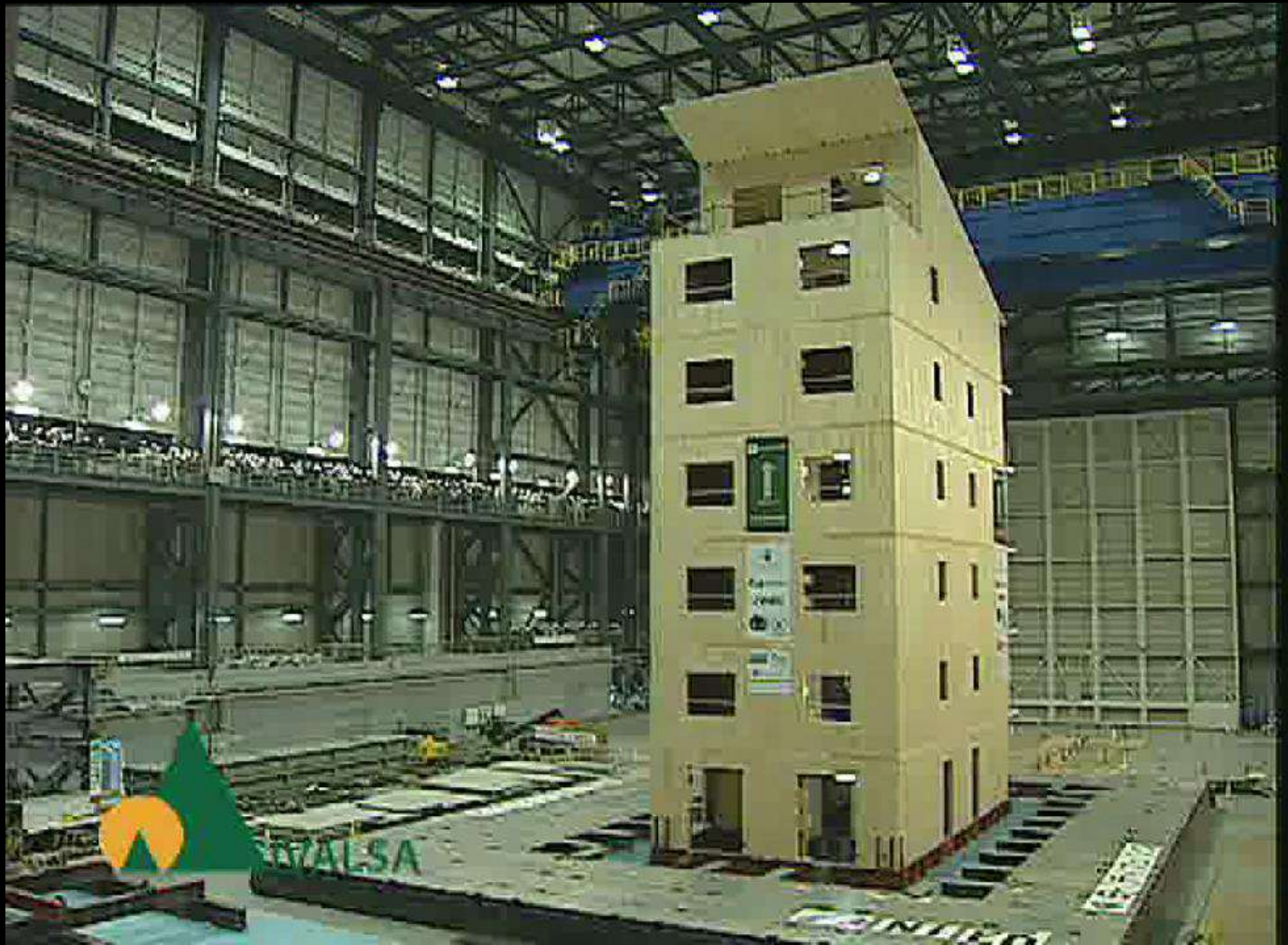
Seismic Test In Miki of a CLT System Building
