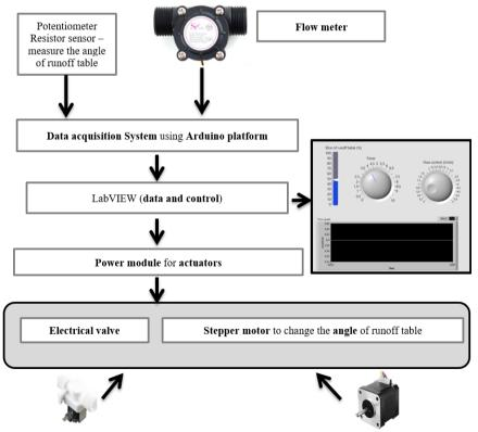
Shape 6. Block diagram of physical computing for runoff table artefact
