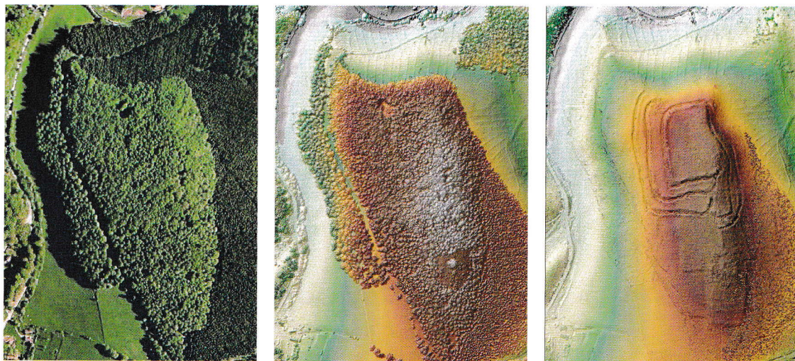
3.22 LiDAR in operation: (left) the Iron Age hillfort of Welshbury in the Forest of Dean, England, is almost invisible in conventional aerial photographs. (Center) The initial LiDAR image shows little improvement but, once reflections from leaves and trees (the “first return”) have been filtered out using a software algorithm (right), the earthworks are clearly visible.
