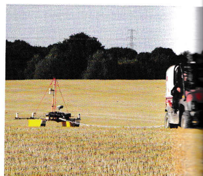
3.51 (Top) The Bartington Grad 601-2 single axis, vertical component, high-stability fluxgate gradiometer system.
