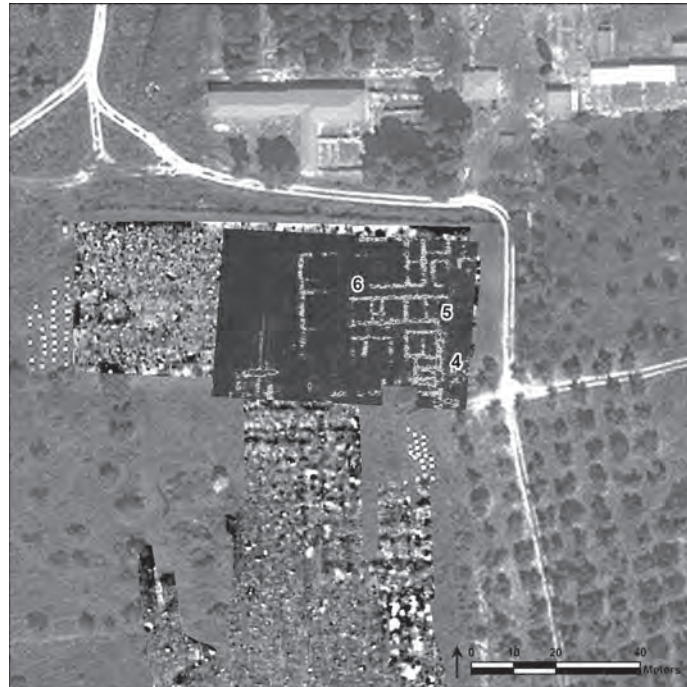
Fig. 7. Demetrias: results of the GPR survey using a single channel 250 MHz antenna (depth: 1.30-1.40 m) south of the palace superimposed over the magnetics survey.
