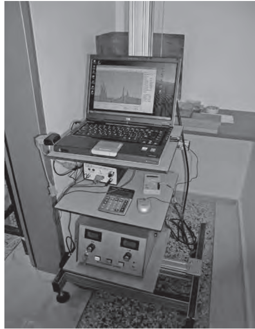
Fig. 15. XRF device used for the analysis of the bronze coins.
