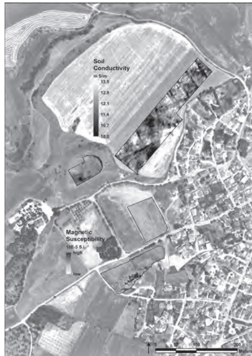
Fig. 3. Pherai: results of the electromagnetics survey both for the electrical conductivity (northern region) and magnetic susceptibility (southern region).
