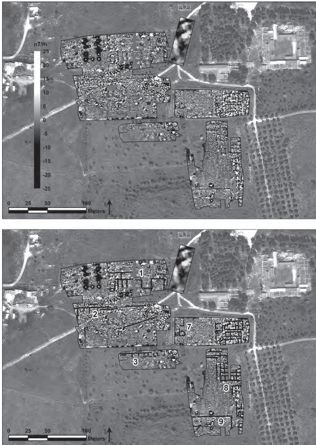
Fig. 6. Demetrias: top , results of the magnetics and electrical ground resistance survey in the regions west and south of the palace; bottom , interpretation of the magnetics survey.
