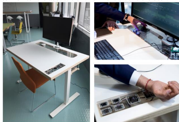
Figure 3: Version 2 of the desk (left), Wireless charging (top-right), and RFID sensor (bottom-right)
