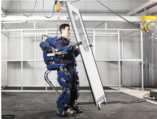
Figure 15 A Hyundai wearable robot, or exoskeleton, relieving workers' fatigue by carrying of the weight. Credit: Engadget
