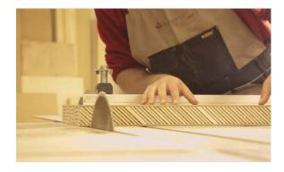
There is no need for special equipment to process DendroLight® door blanks. They can be processed as easy as plywood, MDF or HDF.
