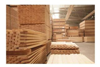
DendroLight® door blanks must be stored on leveled ground on wooden supports or pallets with frequency that does not allow blank bending. Always use cover sheets while storing the blanks in a warehouse. If several blanks are placed on top of each other, wooden supports must form a vertical line.
