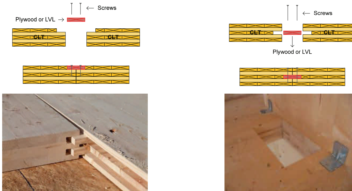
Figure 7. Examples of Types of Connections Typically Used to Establish Panel to Panel and Wall to Floor Connections in CLT Assemblies
