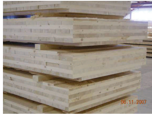
Figure 1. CLT Panel Configuration
