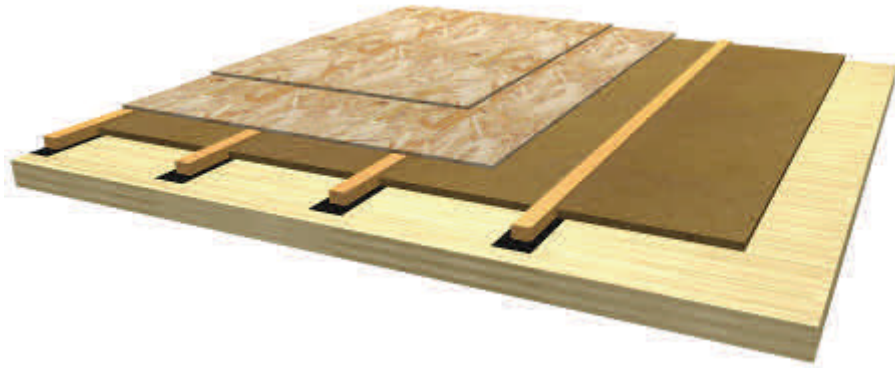
Figure 8 CLT Floor Sound-Insulated on the Top
