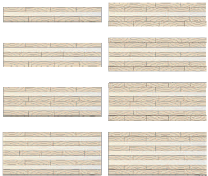
Figure 2. Examples of CLT Panel Cross-Sections
