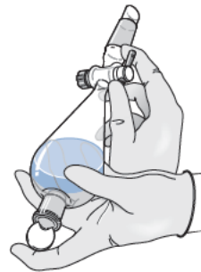
4. Invert funnel and immediately open stopcock to release pressure, close the stopcock, and mix the layers by shaking the funnel.
