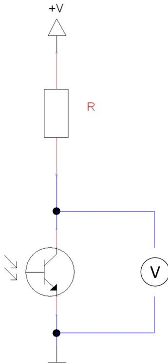
If you switch a resistor and a transistor in row, you will see a special behavior if you measure the voltage at the transistor: if much light shines at the transistor, you will measure a very low voltage (near 0V). If the transistor stays in the dark, you will measure a voltage near +V.
