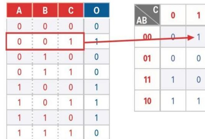
The truth table shows the relationship between four variables (A, B, C, O). The Karnaugh map shows the same data in a Gray-coded format where adjacent cells differ by only one bit.
