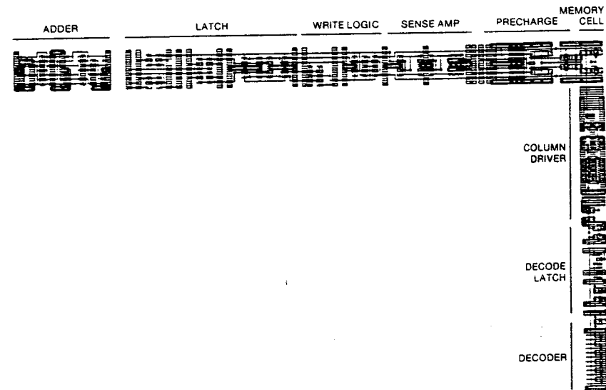
FIGURE 9.80. Layout of a vertical slice through the memory module, and of portion of ALU pitch-matched to a memory cell
