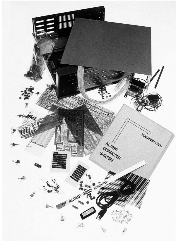
The MITS Altair 8800, unassembled: Early purchasers of the MITS Altair received a bag of parts and assembly instructions. (Courtesy of David Bunnell)
