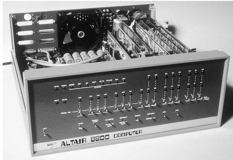
The MITS Altair 8800, assembled: The default input and output for the Altair computer were the switches and lights on the front panel. (Courtesy of Intel Corp.)
