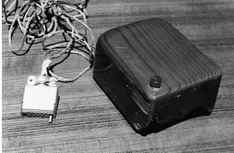
The first mouse: Douglas Engelbart invented the mouse in 1964 as an input device. This first one was carved from a block of wood. (Courtesy of Doug Engelbart)
