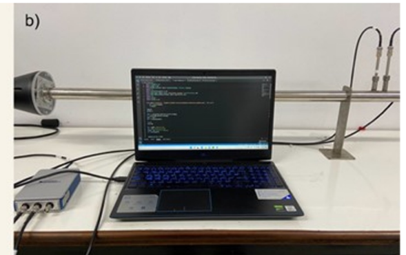
Diagram of the cylindrical two-microphone impedance tube and b) the image of the impedance tube setup used in the measurement
