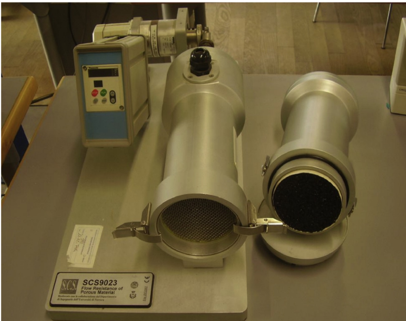
Kundt's tube for the absorption coefficient measure (above) and airflow resistance measurement system at alternate airflow (below)
