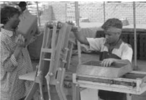
Compressed earth bricks being produced in Gujarat
