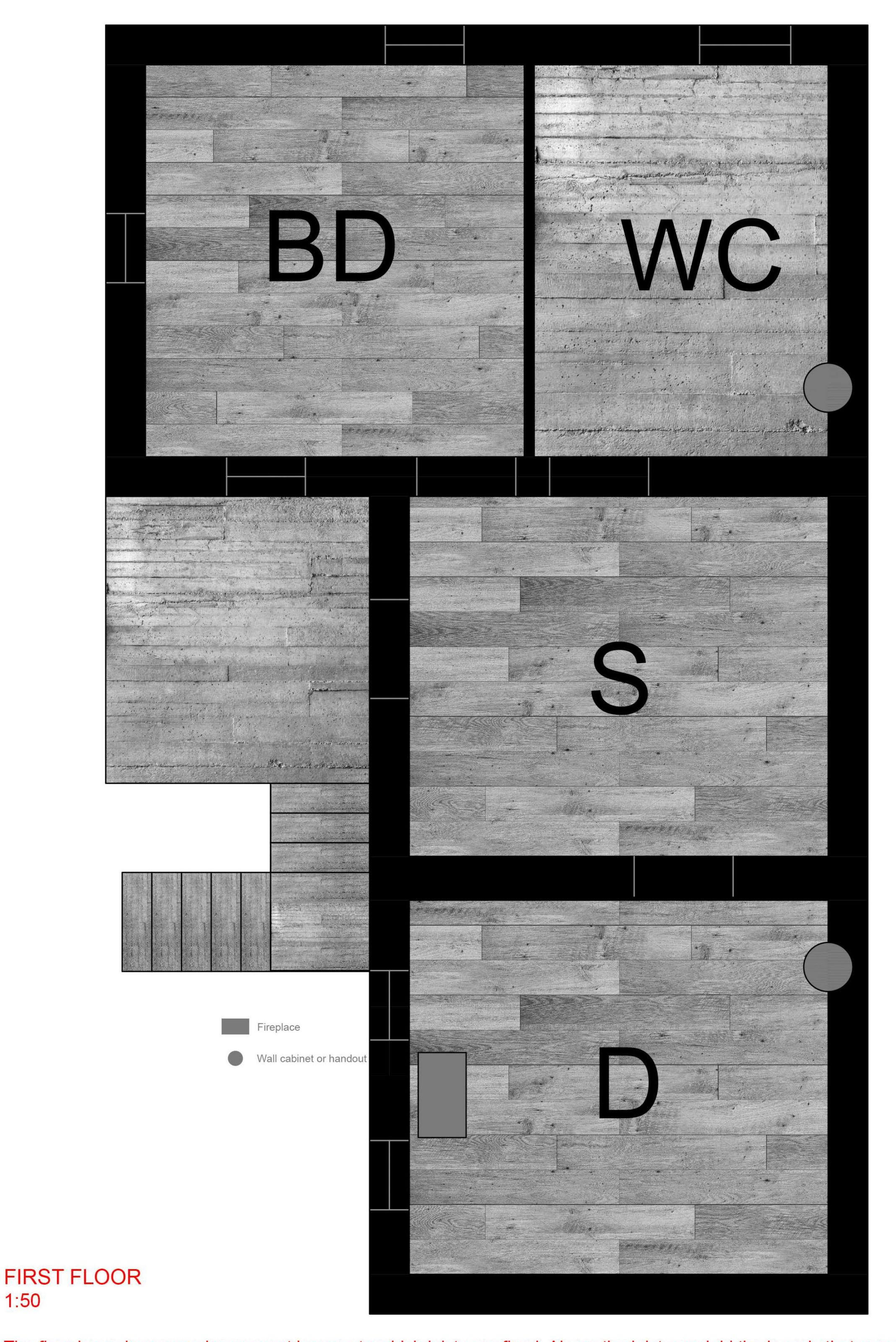
The floor is made on wooden support beams, to which joists are fixed. Above the joists are laid the boards that constitute the flooring. There are no sound-absorbing materials and no pipes run through, only electricity cables. The use of concrete in only one room suggests that is the bathroom, but the lack of toilets and sinks cannot confirm the suggestion.
