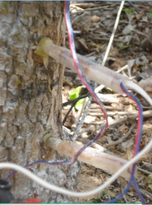
Tree sap flow sensors. 36 trees were measured continuously
