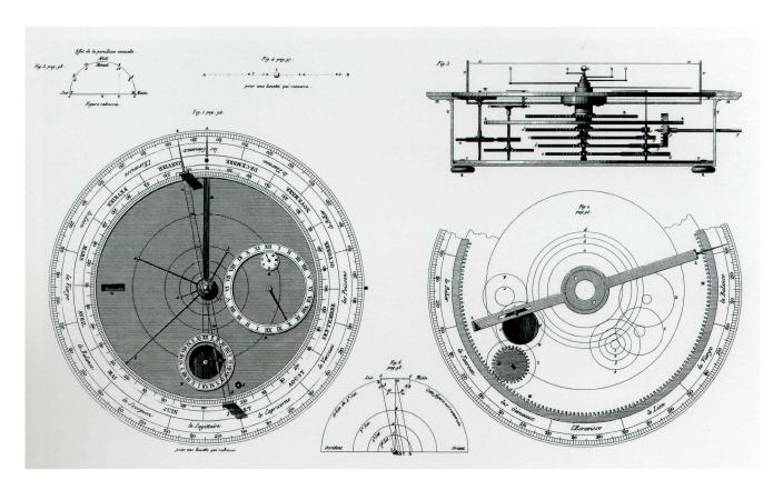
To animate flatland, Galileo and then others constructed Jovilabes, nomogram-like computation devices that recounted orbits of Jupiter's satellites (above). Mechanical models of the solar system in motion showed the interplay of Sun, Earth, and Jupiter, as our shifting vantage point and Jovian shadows masked Galilean satellites from Earth view.
