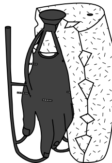
8. Bronze has been poured, investment mold partially broken away.
