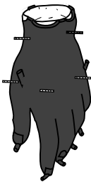
9. Cast bronze hand with core, chaplets and clipped gate system.
