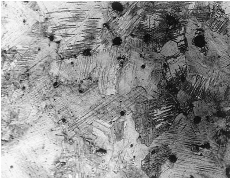
FIGURE A3. Horse, sample no. 1. Metallographic surface section, magnified 300 \times , illustrating the final intensely polished cold-worked microstructure. Photo by Dr. H. Andreopoulou-Mangou.
