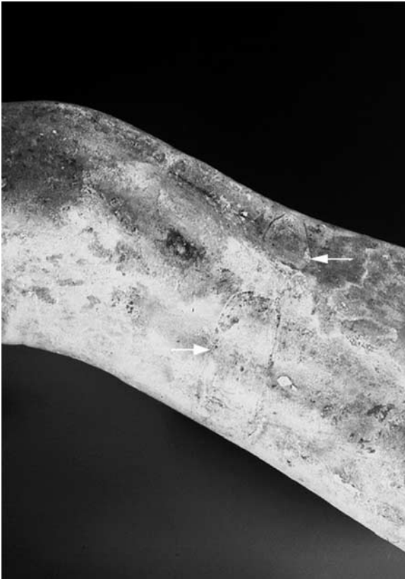
FIGURE 43. Detail of outer left foreleg of the Artemision Horse. Arrows point to ovals of flow weld. Photo by the author.
