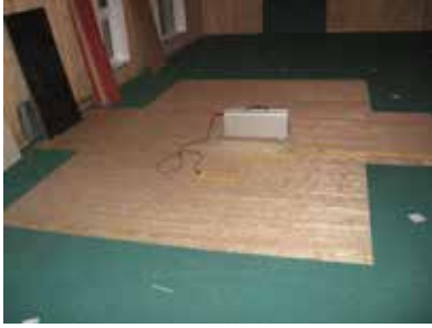
(a) Source room with the tapping machine on the floor in a field floor/ceiling assembly
