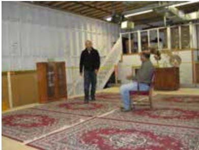
Figure 6 CLT floor built in laboratory for the vibration tests and subjective evaluation
