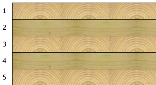
Figure 6 Cross-section of a 5-layer CLT panel
