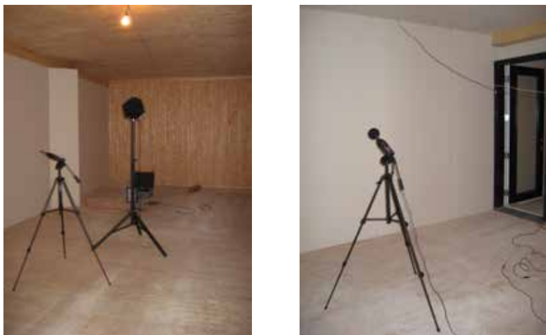
(a) Source room with an omnidirectional loudspeaker as the source and a sound level meter (b) Receiving room with a sound level meter to measure the sound transmitted through the wall
