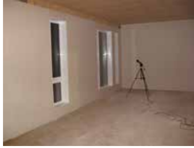
(b) Receiving room under the source room with a sound level meter to measure the impact sound transmitted through the floor/ceiling assembly
