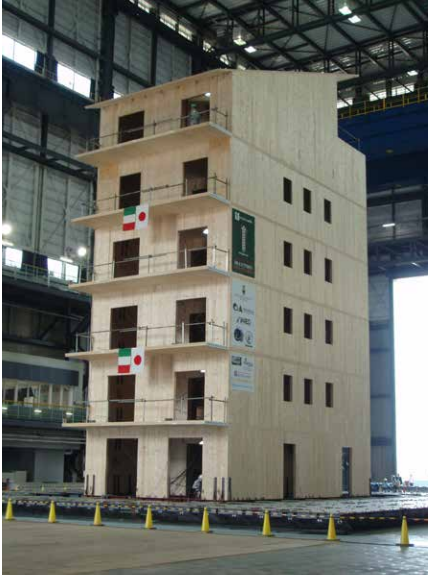
Figure 8 Seven-story CLT building tested at E-Defense Laboratory in Miki as a part of the SOFIE Project and CLT test assembly at FPInnovations
