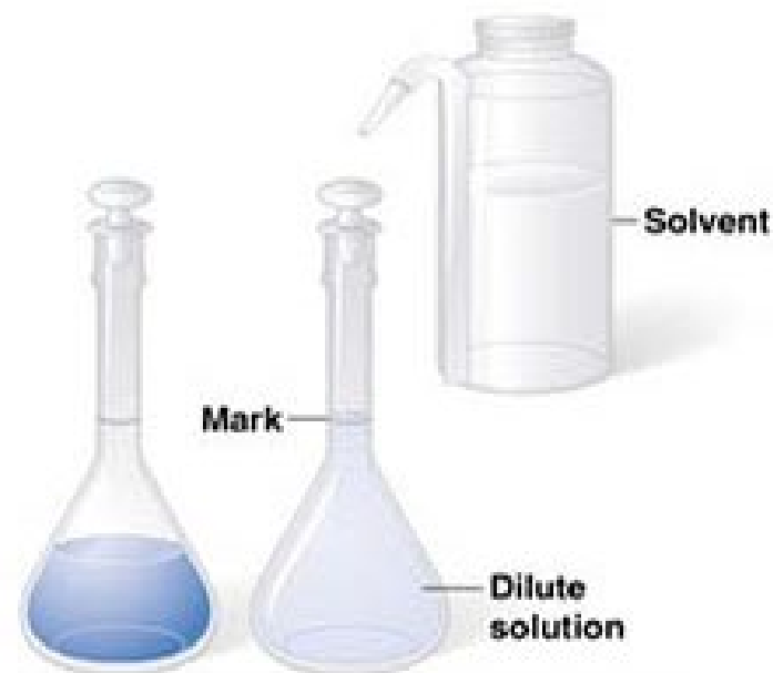
(c) The measured volume in the second flask is then diluted with solvent up to the volumetric mark [ (V_s)(M_s) = (V_d)(M_d) ].
