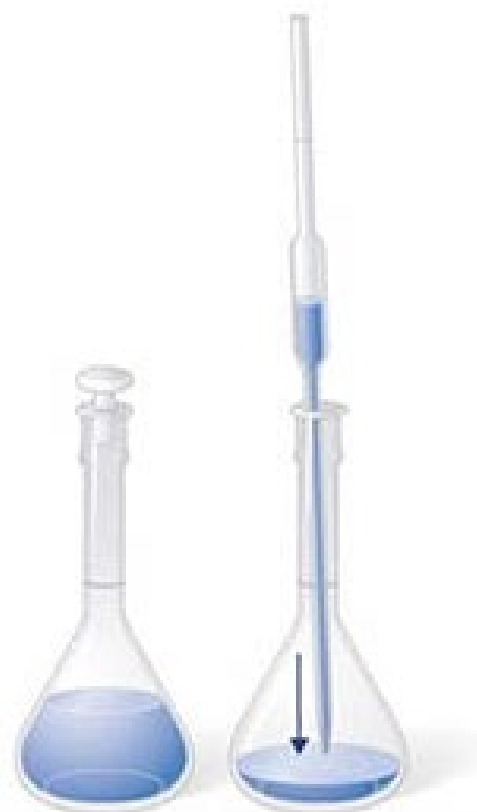
(b) The measured volume of stock solution is transferred to a second volumetric flask.
