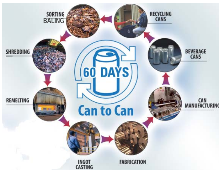
Figure 27: The recycling process of aluminium cans
