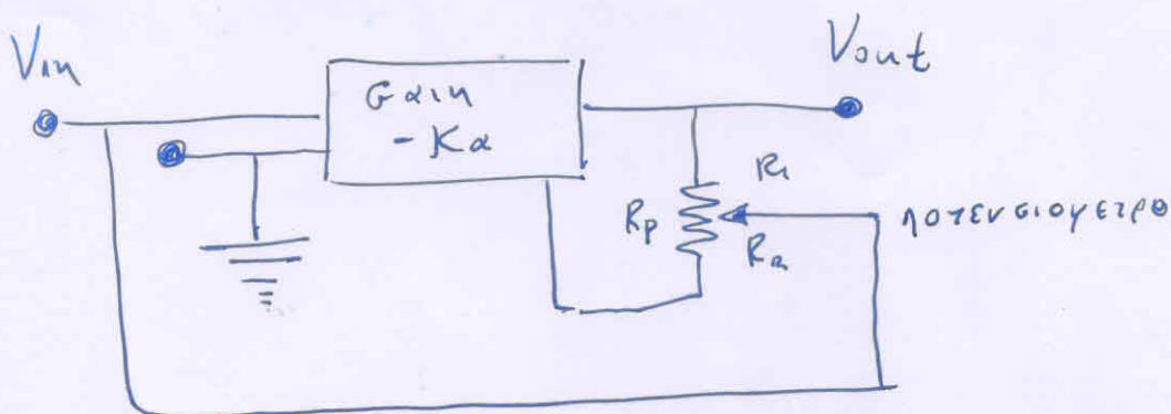
$$V_{out} = V_{out}(s) = -K_\alpha V_{in}(s)$$
