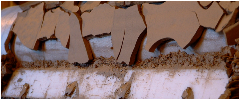
Figure 8: Positive cake discharge on a belt filter (Outotec Filters). The change in direction as the cloth passes over the roller causes most of the cake to fall, with a scraper providing a back-up.
