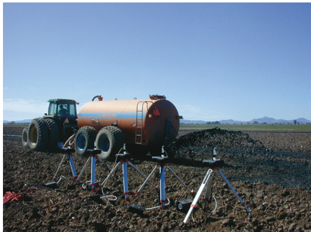
FIGURE 5.12 Land application of liquid biosolids via a spray application, and collection of air samples via biosamplers.
