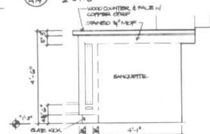
13 EAST ELEVATION OF CASHIER STATION A14 2' = 1'-0"
