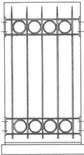
Grille, with ornament between bars, set in masonry opening.
