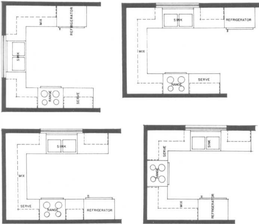
Fig. 4 U-shaped plans. If dishwasher is desired, it should be located at sink center.
