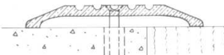
Threshold fastened with screw in fibre plug or expansive metal anchor. Floor may be cement, terrazzo or similar construction.
