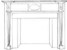
CHIMNEY PIECE IN THE STYLE OF SAMUEL MCINTIRE SHELF 5-11/2" WIDE, 4-0" HIGH WOOD OPENING 3-8" WIDE, 3-0" HIGH WIDTH MIDWAY 4-11" 4" PROJECTION
