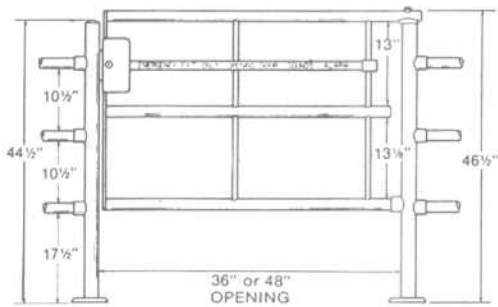
Triple rail — alarm system
