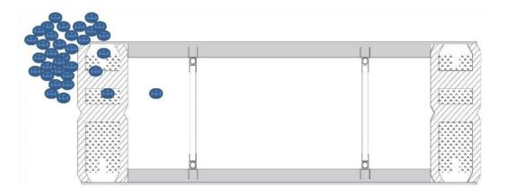
This means that elastic seals can be used which are not only cheaper and easier to process than glass/metal seals, for example, but can also compensate for different material expansions.
